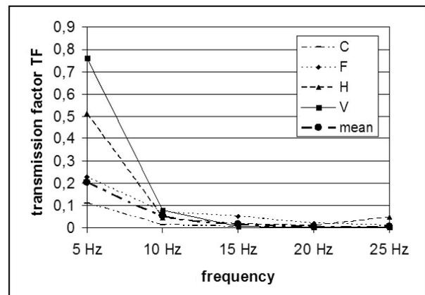
Fig. 2: Transmission factors [RMS head/platform]
